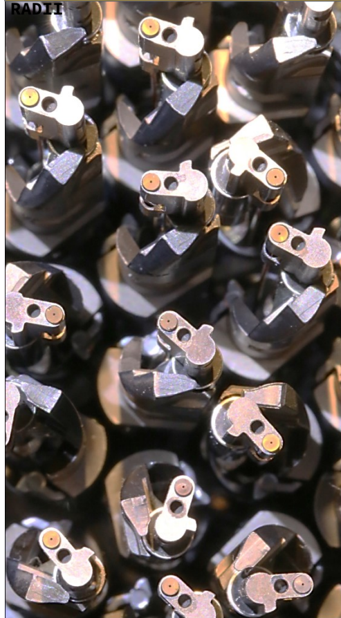
DESI FIBER ROBOTS ARRAY, 10.5 mm PITCH, OVERLAPPING PATROL RADIUS
