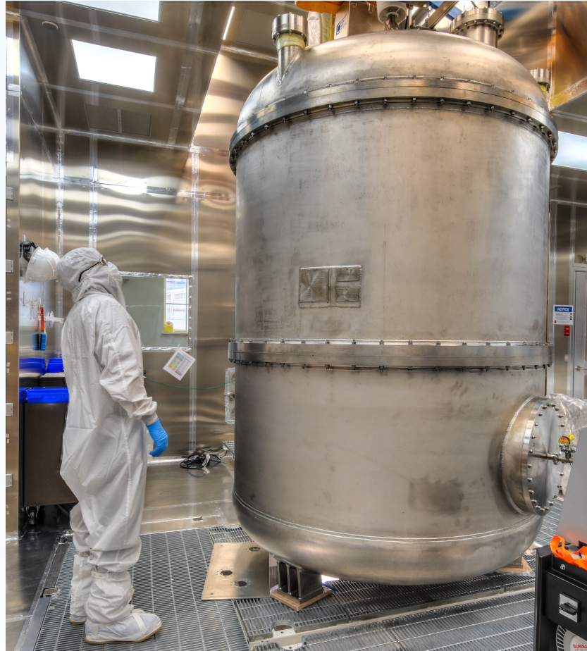
Leak checking the outer cryostat in the surface cleanroom
