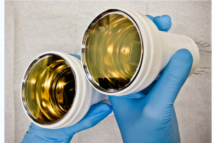
A pair of LZ photomultiplier tubes (PMTs)
