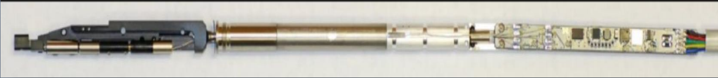
5,020 phi-theta fiber positioners, 10.4 mm, 12 mm patrol region
