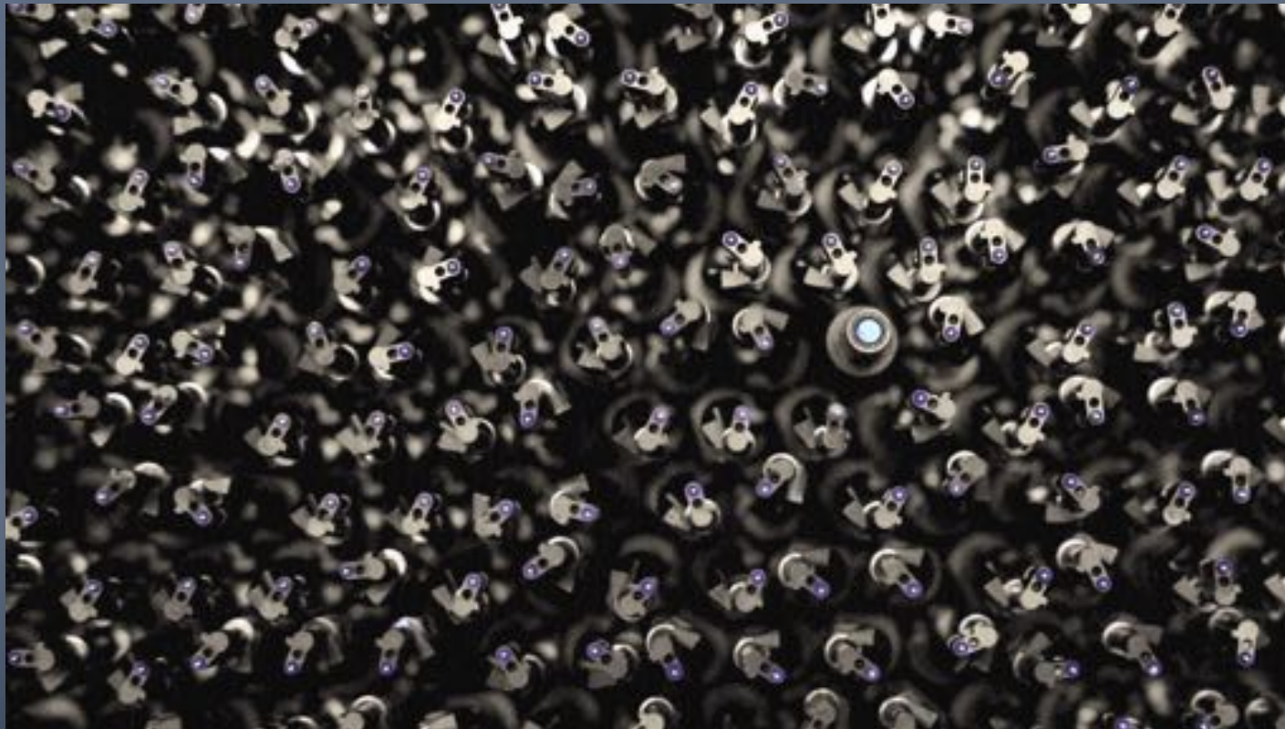
5,020 phi-theta fiber positioners, 10.4 mm, 12 mm patrol region
